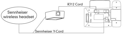
**Note:** The sennheiser wireless headset must be the latest firmware of the DW-Office series (version 96 or later) !
